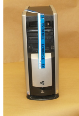
Seal the front with evidence tape as well to prevent any of the drives being opened.
