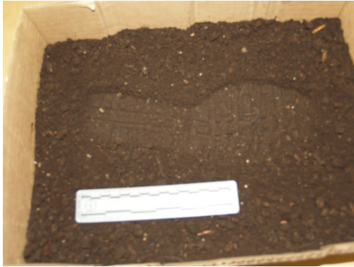
Photograph the impression with a scale at a 90° with a scale in the photo.
