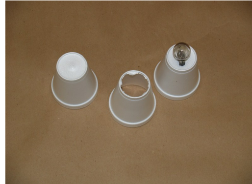
Push bulb through a hole cut into the bottom of a cup. Cut the bottom out of a second cup. Leave the third cup as is.
