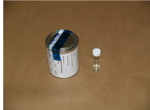
Liquids should be no more than 2 ml and placed in a friction lid can filled with an absorbent material.
