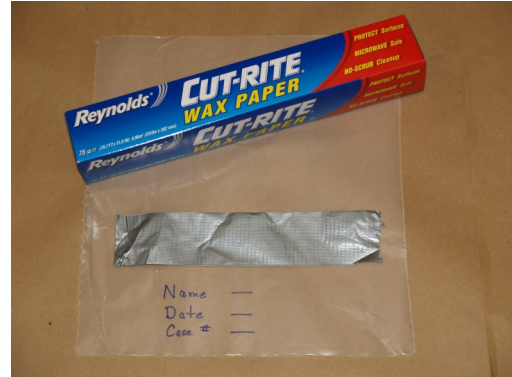
Place sticky side down on wax paper or heavy plastic. Mark wax paper with identifiers. Wrap wadded tape in wax paper.
