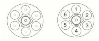
Scratch arrow on rear face of cylinder to indicate the chamber position under hammer (inline with barrel), when recovered. Then prepare diagram numbering in clockwise direction the remaining chambers, i.e., 2.3.4.5.6. etc.
